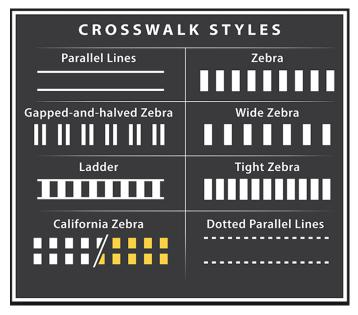
Crosswalks are marked at intersections where there is substantial conflict vehicle pedestrian between and movements, where significant pedestrian concentrations occur, where pedestrians could not otherwise recognize the proper and where traffic place to cross. movements are controlled. Examples of such locations are:
