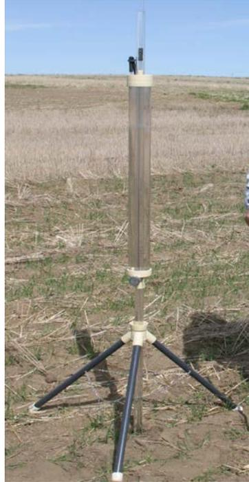
Figure C-3: Guelph Permeameter for Shallow Borehole Permeability
