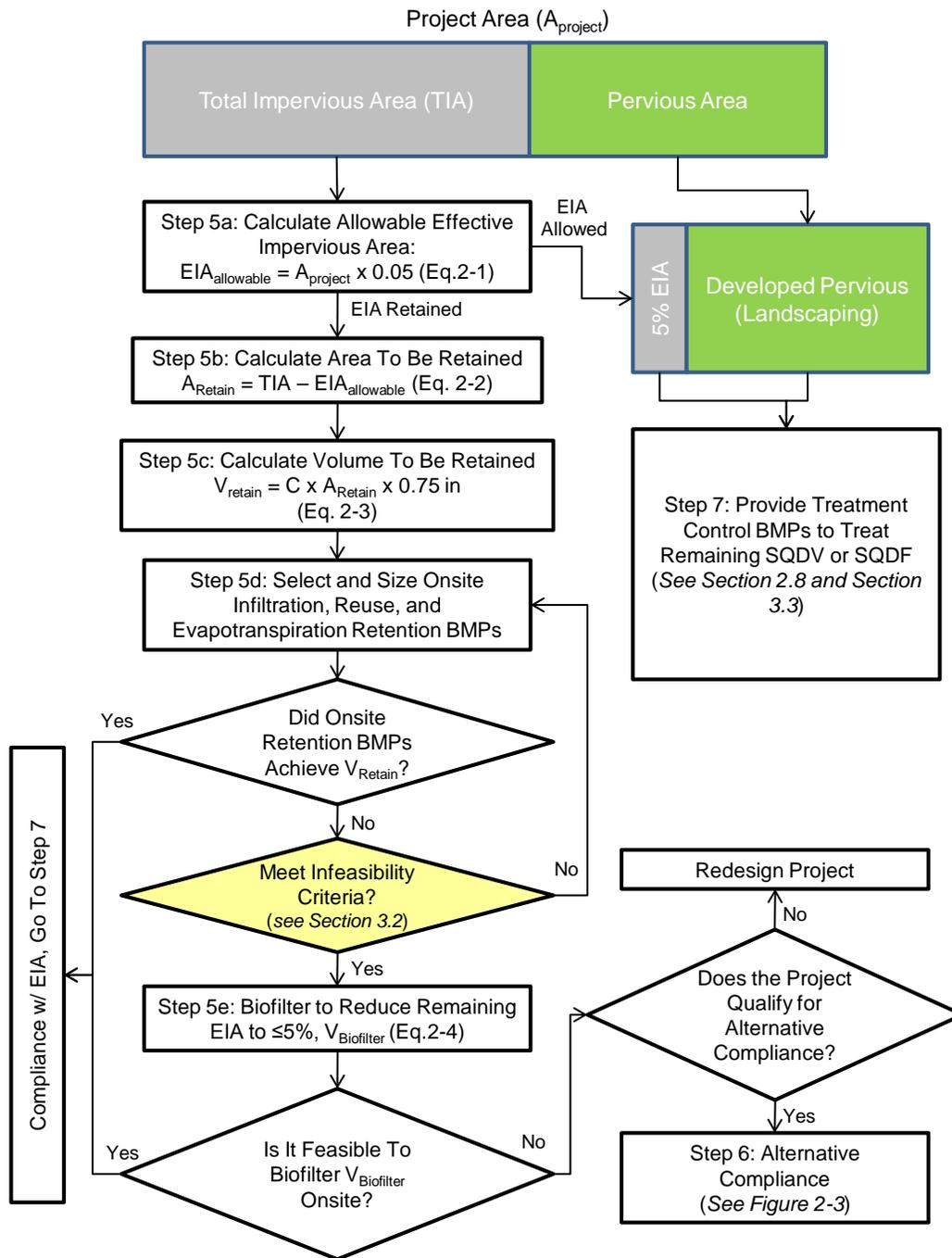
Figure 2-2: Apply BMPs to Reduce EIA to  $\leq 5\%$  Process Flow Chart
