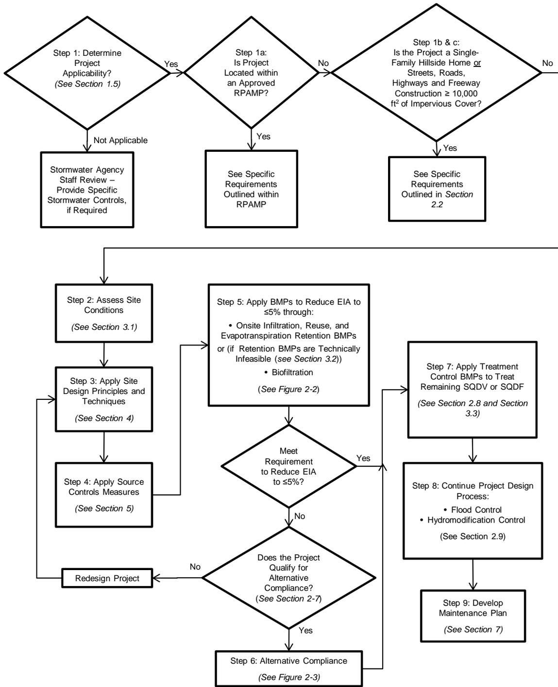
Figure 2-1: Stormwater Management Control Measures Design Decision Flowchart
