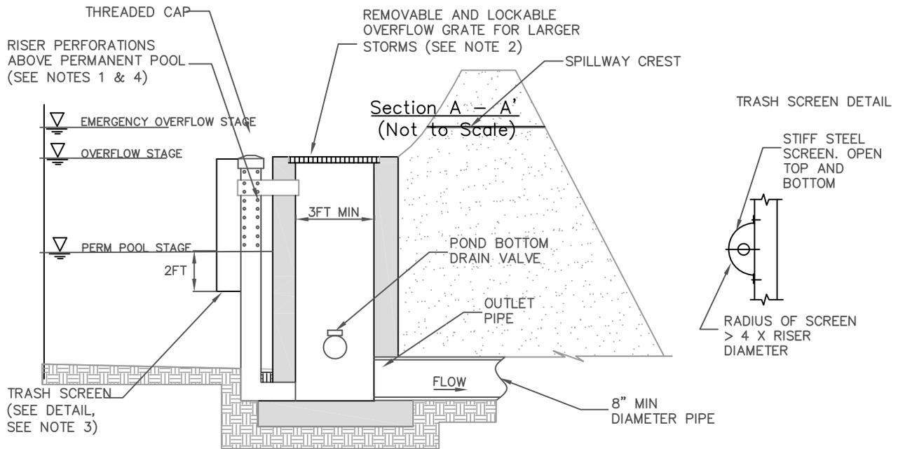
Perforated Riser Outlet Structure
