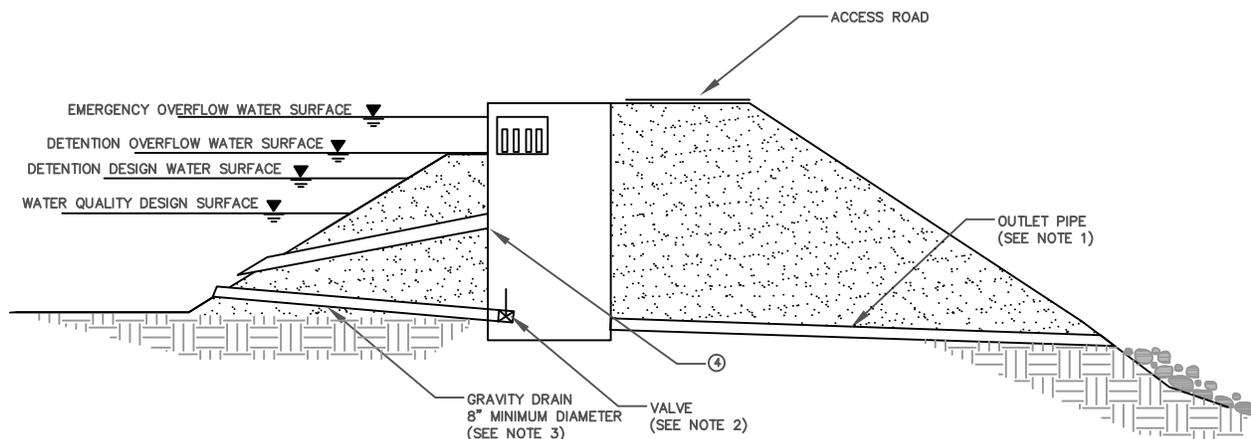
Inverted Pipe Outlet Structure
