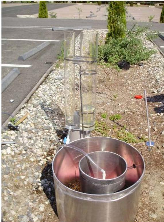
**Figure C-2: Double Ring Infiltrometer**
