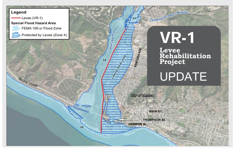
The VR-1 improvements consists of upgrading the levee system beginning at its downstream end at the Pacific Ocean and extending upstream along the Ventura River to its upstream end downstream of Canada de San Joaquin. The overall length of the levee is approximately 2.65 miles, with an embankment height up to 10 feet above natural ground on the landward side.
